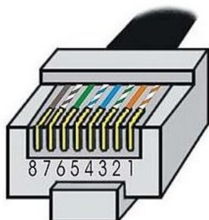
Fig 5.1 Pin Configuration for standard RJ45 plug
