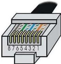
Fig 7.1 Pin Configuration for standard Type T-568B RJ45 plug
