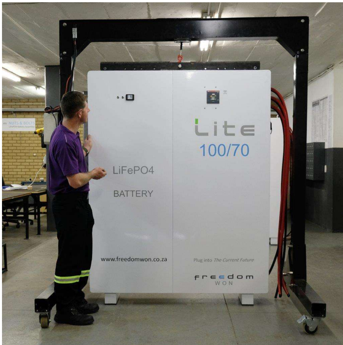
Fig 3.5 Site Assembled Gantry with Electric Winch
