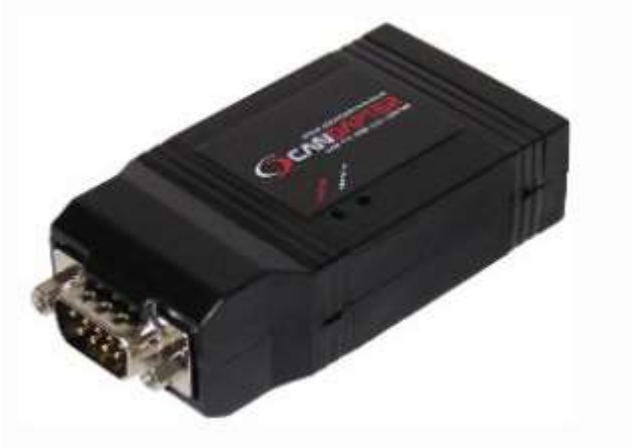
Figure 2.4 CANdapter for Programming Freedom Lite Commercial Range
