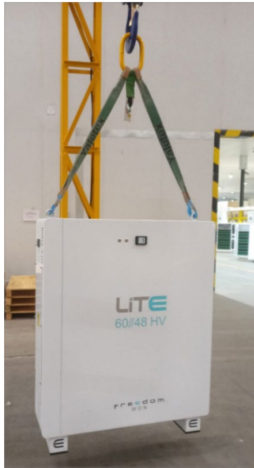
Figure 3: Lifting and Handling Example
