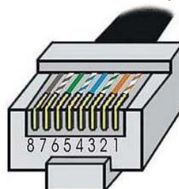
Fig 6.1 Pin Configuration for standard Type T-568B RJ45 plug.
